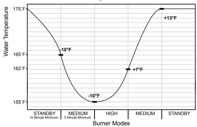
If burner temperature is not high enough the controller will not switch from MEDIUM to HIGH mode.
